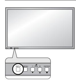
Press the INPUT button to select the input signal to be played back from the equipment which has been connected to the Plasma Display.
